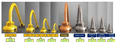
Microchip's wire bonding process development
